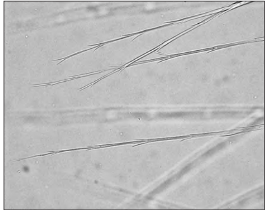
Figure 4. Photomicrograph of downy barbules of American white pelican ( Pelecanus erythrorhynchos ) showing the microscopic similarity to the unknown sample (Figure 3) from the Wiley Post accident.
